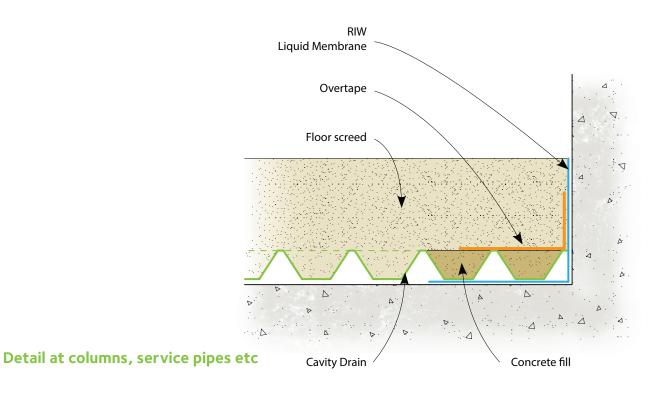
All overlaps: Should be sealed using a run of Sealing Rope or Tape placed along the flat area of the Cavity Drain membrane between the two rows of domes. It is recommended that if the product is used as a radon barrier, all lap joints must also be sealed internally with Overtape.
