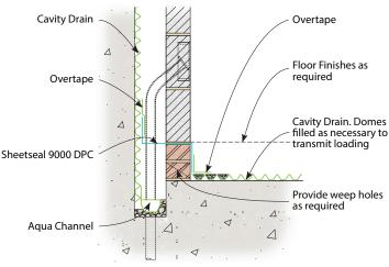
**Wall Floor Junction with Masonry Lining Wall**
