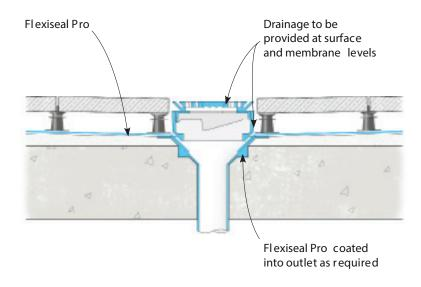
**Typical Details at Drainage Outlet**
