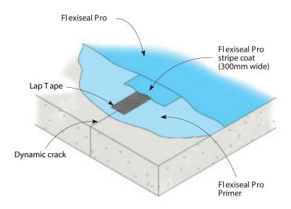
**Detail 4 - Dynamic Crack Bridging**
