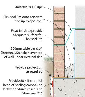
Structureseal peel adhere to concrete, terminated on vertical face at top of wall
